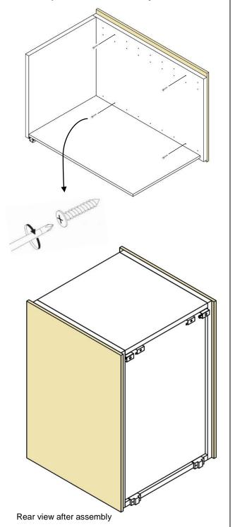
Secure the panel with screws by placing them on the inside of the body.
